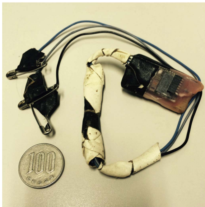
Fig. A.1. Neurologger 2A for ECG (0.625 ms sampling interval, voltage range \pm 3 mV, 20 g weight, 1 GB memory and Li-Po battery of 3.7 V and 240 mAh, Evolocus LLC) and 100 JPY coin (diameter of 22.6 mm). Three wires extending from the ECG logger soldered to small safety pins that are attached subcutaneously to the skin under the feathers, and function as
